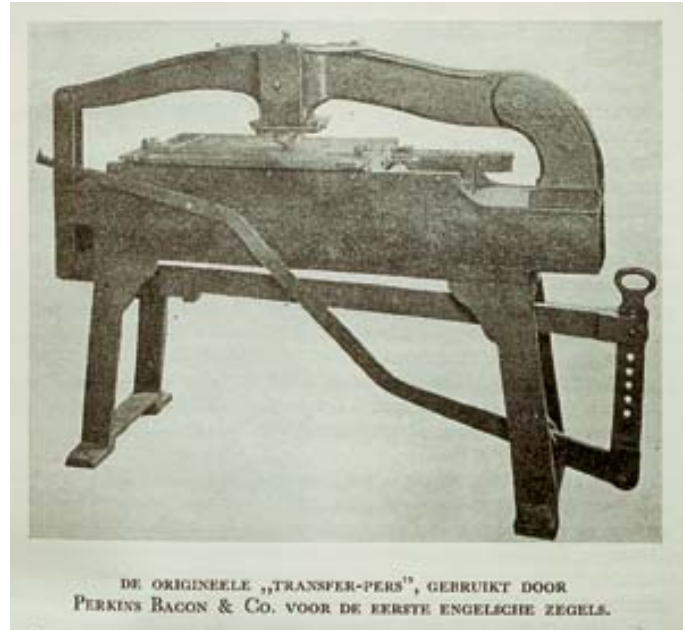
The original transfer press manufactured by the British firm Perkins Bacon & Co. was used to rock the die into the plate—stamp by stamp.
