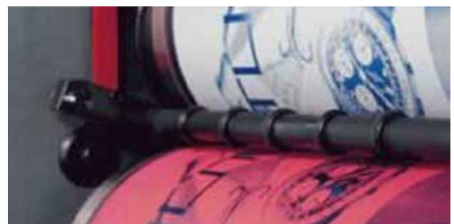
The blue ink on a white background is the inked offset plate in correct way reading. The blue ink on red area is the design offset on the rubber blanket in reverse way reading.
