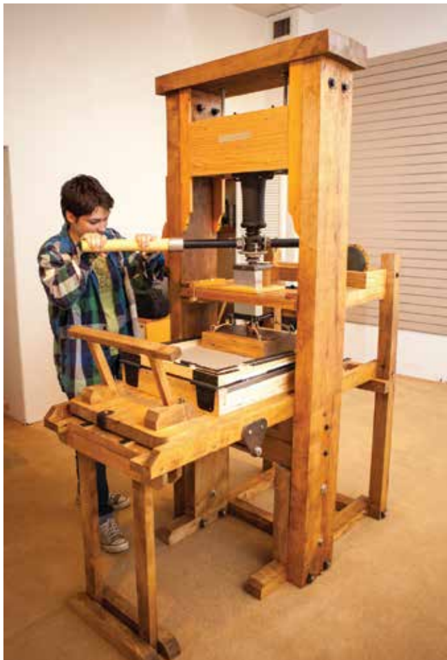
Grace applies pressure to the tympan thereby printing the paper. Photo by Aura Moore.
