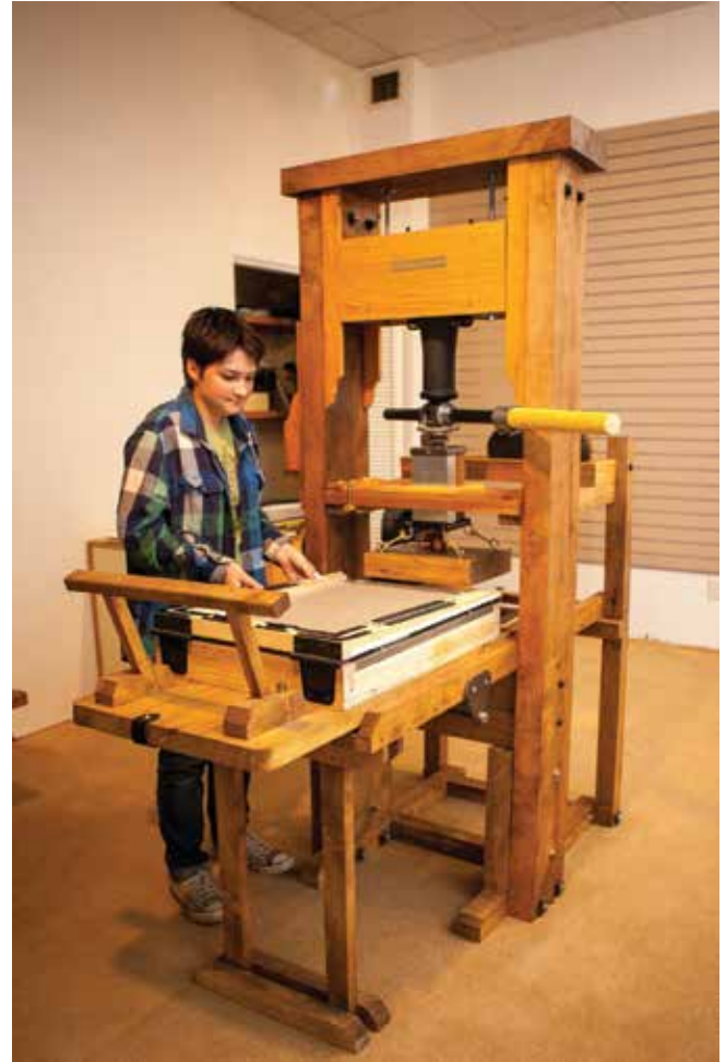
Grace lowers the tympan holding the paper onto the inked type. Photo by Aura Moore.
