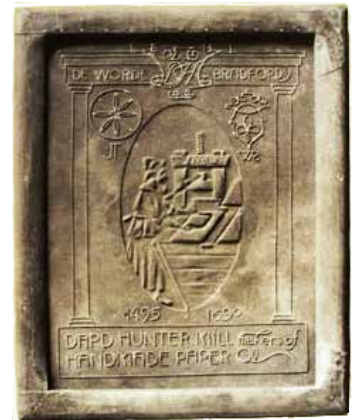
Fig. 3. Combination line and light-and-shade watermark by Hunter sewed to a mould frame made by T.J. Marshall. Mould is 9 1/2" x 12 1/4".
