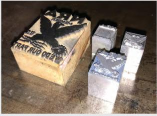
terms). The large plate was etched into a piece of Bakelite (plastic) which is unusual, as most plates at that time were etched into a sheet of zinc or copper and mounted on a wood base.
