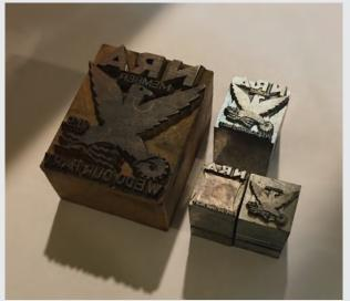
Printing plates used to produce the NRA "Blue Eagle" from the author's collection. The two small plates were used to print the two-color label. They are about ½ inch square (36 points in printers'
